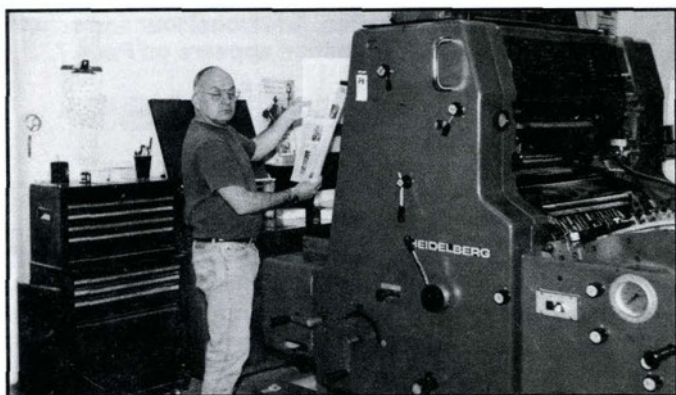
HEIDELBERG might sound like one of our WW II targets, but that's the German city where the big press comes from that prints FLAK NEWS. This is a single color, offset sheet-fed press that turns out 6,000 impressions per hour. Ron, Nils, Perry and Rob operate this and other presses at Vanguard.
